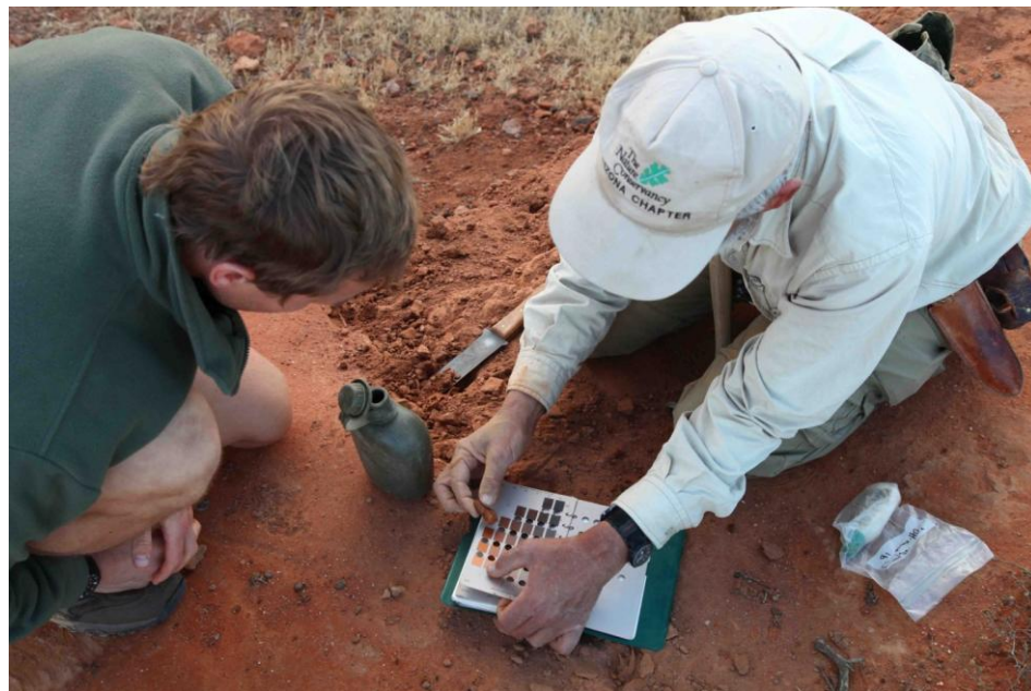
Joe explaining the use of a soil colour chart to Wesley. The percentage of sands to silts and clays is also tested by wetting the soil, forming it into a ball, and then feeling for texture and clay content by pushing the soil into a ribbon between two fingers.
