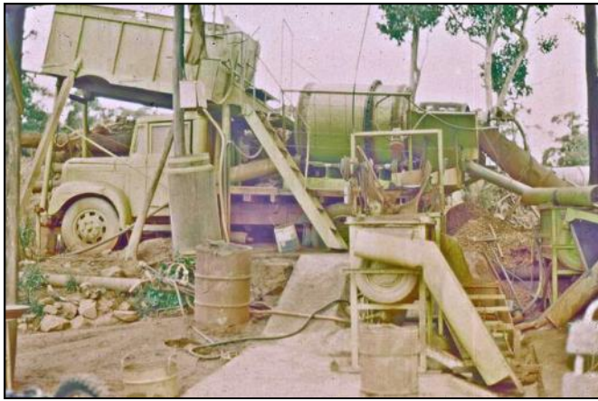
14. The Morris Commercial truck as it was in May 1981, complete with trommel (rotating drum with screens inside). Note further concentrating equipment in foreground.
