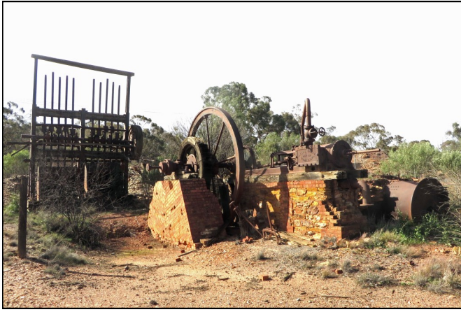
63. The 1897 Barrass and Conley 10 head stamper and steam engine on the Golden Walk at the Peak mine.
