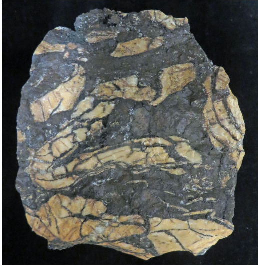
37. Slump bedding in chert from the Whip Shaft, Nymagee mine. 10 cm.
