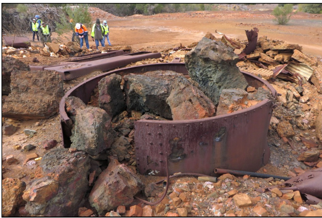
28. Bosh ring from the blast furnace filled with broken up slag.
