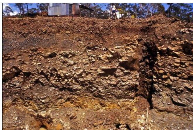
9. December 1981. Open cut mine (view to east from near cliff edge). The deep lead gravels can be seen just above the water filled previous tunnel at lower left of photo (at the base of the basalt). Note the previous shaft on the right of photo (and man on top for scale).
