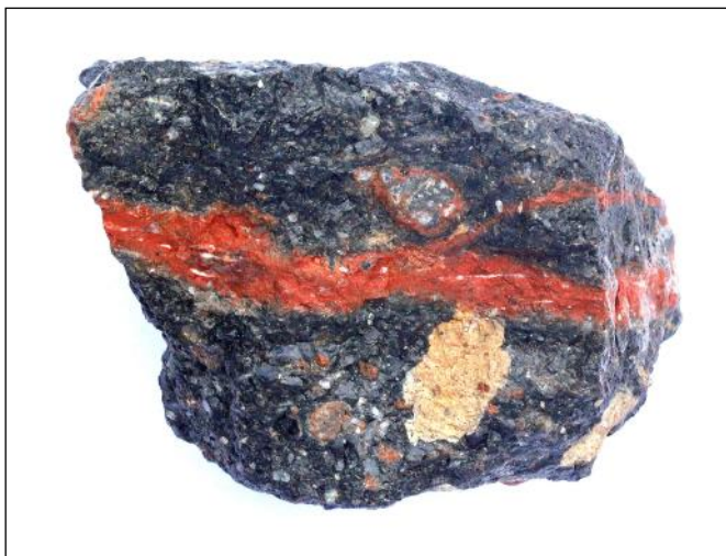
Glassy phase of Lambs Valley Ignimbrite - devitrification occurring. Specimen is 7 cm wide by 5 cm high. (BME specimen R849).
