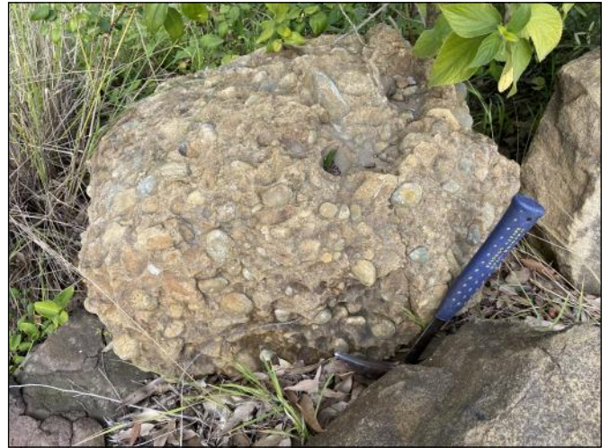
28. Sample of Seaham Conglomerate composed of rounded pebbles within a sandy matrix.
