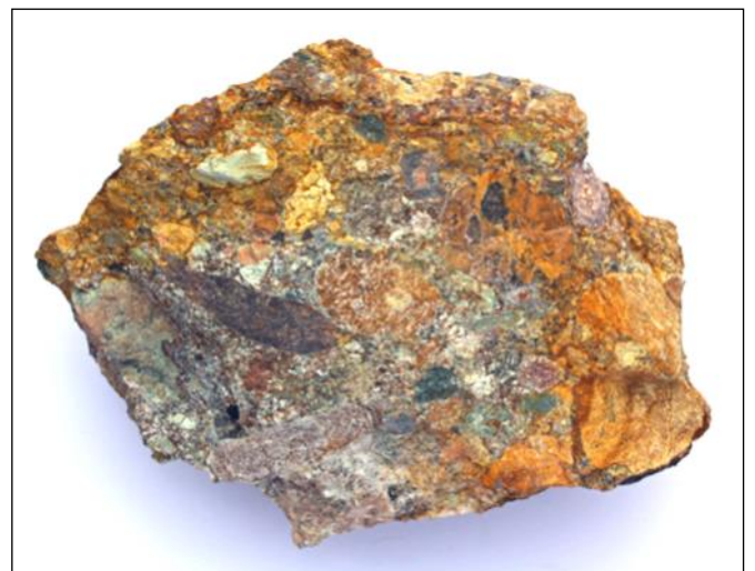
8. Polymictic conglomerate from the Ravensfield Sandstone Member. The rock is very hard probably due to its calcareous cement. Its origin is shallow marine as evidenced by fossils ( polypora , fenestella and brachiopod fragments) found in some samples.
