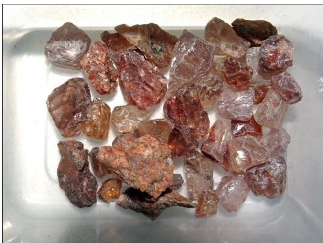
3. Samples of zircon ( ZrSiO_4 ) crystals. These can be used to date a rock by measuring radioactive decay of U and Th to Pb within the crystals.
