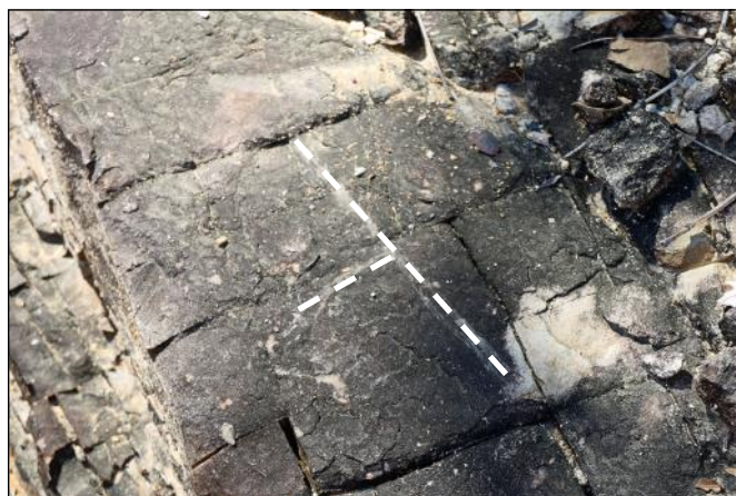
Dip (angle down from the horizontal) and strike (compass direction) as demonstrated by one measurement.
