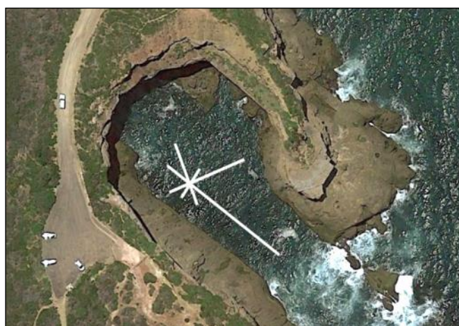
6. The white lines show the direction and persistence (length) of four important joint sets. (Peter Mitchell)
