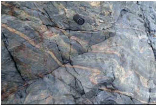
32. Dyke rock is magnetic (due to magnetite) as shown by a magnet within the film canister.
