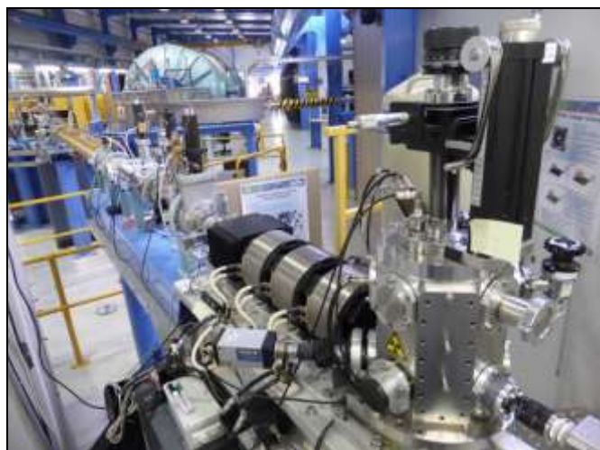
2. 10 MV ANTARES Tandem Accelerator, first commissioned in 1991.
